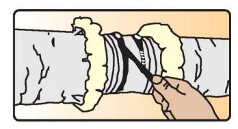
Use atleast 2 wraps of duct tape to tape the jacket. Secure the connection with clamp placed over the core and tape and past the bead.
