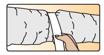
Pull jacket and insulation back over cores. Use atleast 2 wraps of duct tape to tape the jacket.
