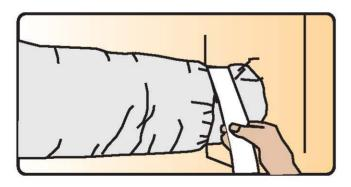
Pull jacket and insulation back over the core. Use atleast 2 wraps of duct tape to tape the jacket. You may use a clamp along with or instead of the duct tape.
