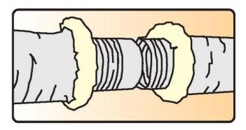
Fold back jacket and insulation from core. Butt 2 cores together on a standard 4" (100mm) length metal sleeve.
