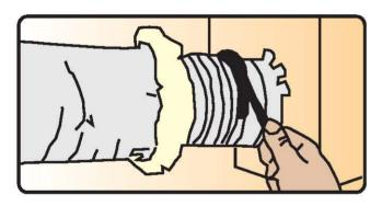
Slide at least 1" (25mm) of core over fitting and past the bead. Seal core to cover with 2 wraps of duct tape. Secure the connection with clamp placed over the core and tape and past the bead.
