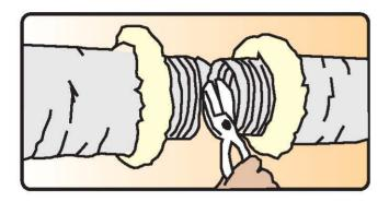
Cut completely around and through the duct with knife or scissors. Cut the wire with wire cutters. Fold back the jacket and insulation
